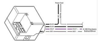
To control multiple ballasts, parallel all ballast input wires (line, neutral and control wires purple and grey). It is recommended to
